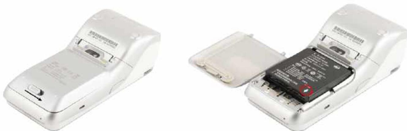
Next lift the battery from the bottom side and swing it upwards from the bottom and pull out.
