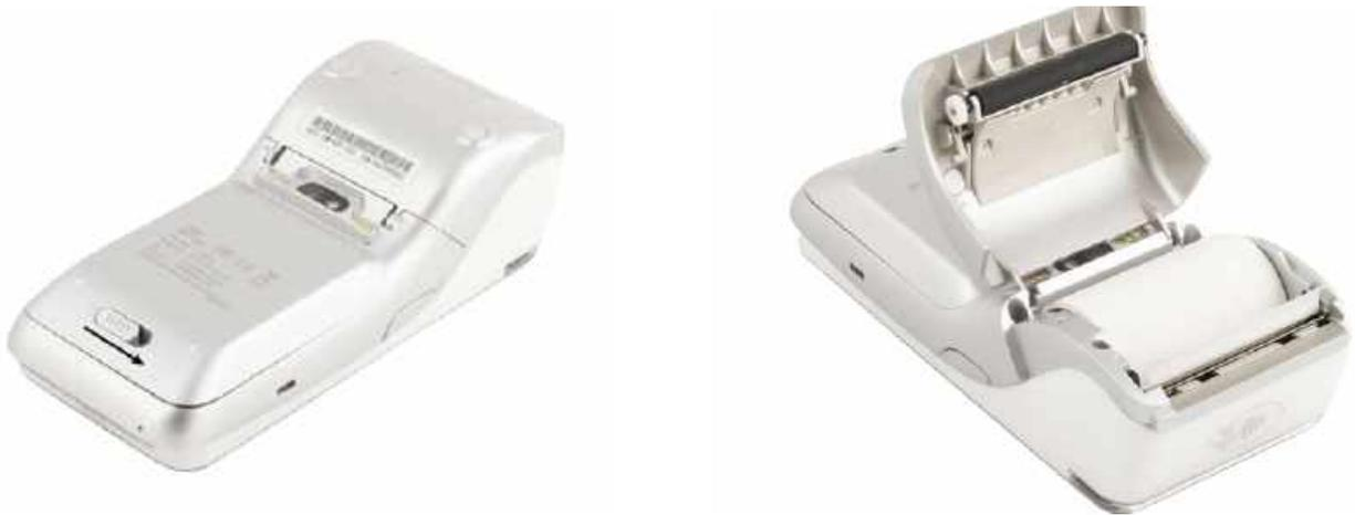
To install a new thermal paper roll, drop in the paper roll with the paper pulling from the back and out the top of the roll. Pull about 2" of paper out and close the lid until the lid snaps into place. It is important the lid is fully closed so that the paper roll fully engages the paper. Tear off any excess paper.
